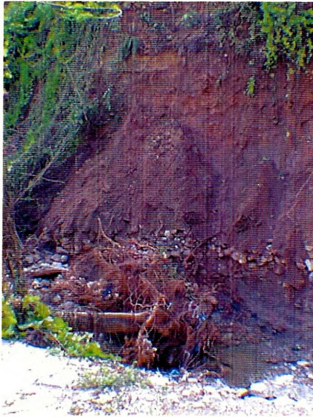
Plate 5. Gully bank slumping destroys retaining wall.
