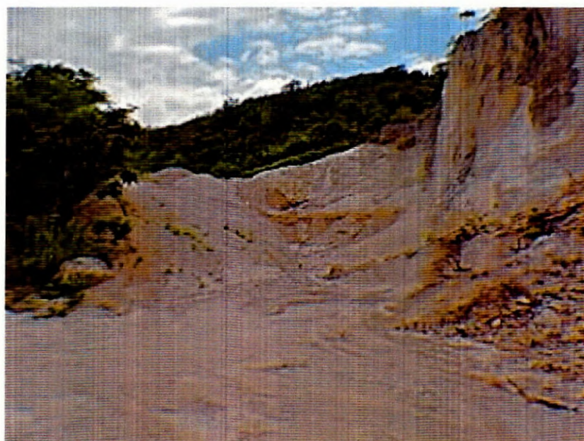
Plate 10. Limestone quarry located 200 feet above Mona reservoir causing debris flow into the Mona Reservoir.
